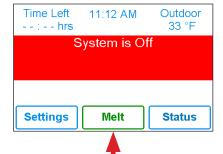
Press Melt button to start melting operation
